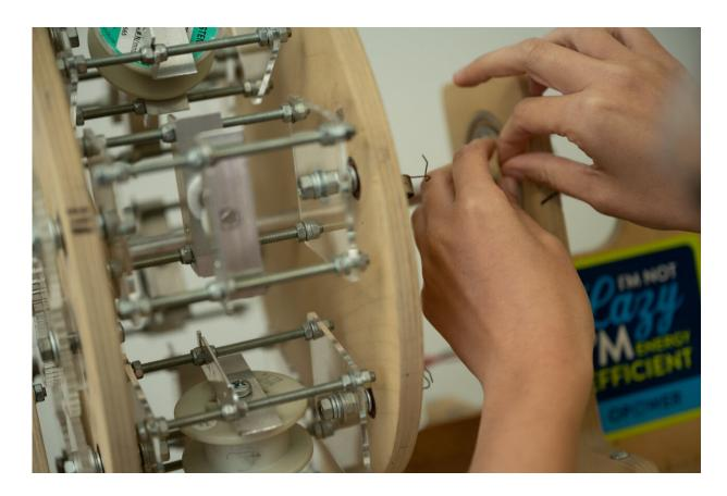
A Rice University lab uses a custom device that weaves carbon nanotube fibers into larger threads for sewing. The threads were then used to make "smart clothing" able to monitor the wearer's heart. Credit: Jeff Fitlow/Rice University
