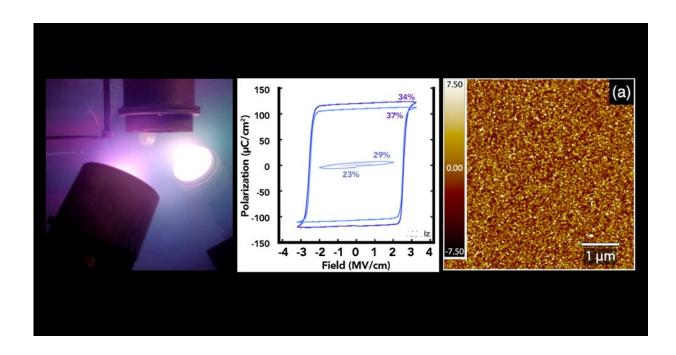
Part of the process of creating ferroelectric magnesium-substituted zinc oxide thin films includes: (left) Image showing thin film being sputter-deposited from metal sources; (center) ferroelectric hysteresis loops of thin-film capacitors showing two remanent polarization states at zero field; (right) atomic force microscope image showing a smooth surface at the nanometer scale and a very fine-grained and fiber-textured microstructure. Credit: Materials Research Institute, Penn State
