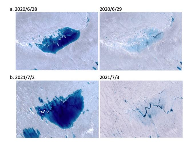
The study used GPS observations of surface uplift caused by lake drainage events. Above, meltwater lakes on the surface (left) empty through fractures in the ice sheet (right). Water from surface melting can act as a lubricant that loosens the ice sheet's grip on the ground. Credit: Sentinel-2
