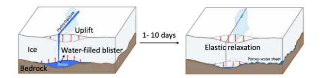
Meltwater-filled cavities push the surface of the ice sheet upward (left), then cause it to gradually drop down (right) as the water permeates the subglacial drainage system. This rise and fall can be used to estimate a property of the subglacial drainage system known as transmissivity. Credit: Ching-Yao Lai, Department of Geosciences
