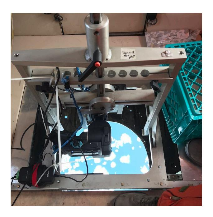
Infrared and DSLR cameras mounted in the belly of the plane look down on sea
