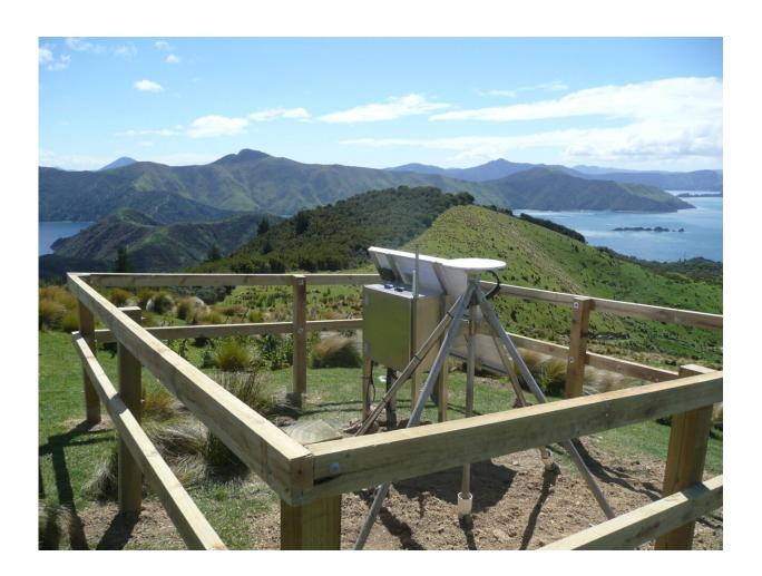
GPS sites like this one in New Zealand continuously monitor changes in the Earth's surface near earthquake hotspots. The new project led by UT Austin is an ambitious physics-driven effort to learn how to spot earthquake warning signs at the world's subduction zones. Credit: GNS Science/EQC
