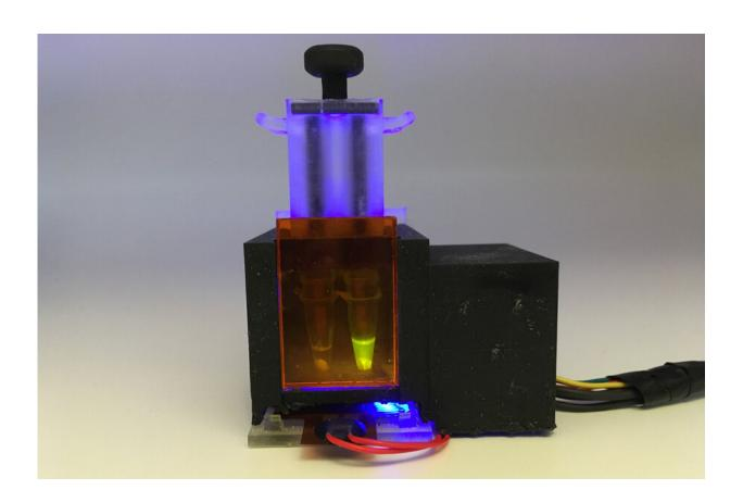
Engineers at MIT and Harvard University have designed a small tabletop device that can detect SARS-CoV-2 from a saliva sample in about an hour. Credit: Devora Najjar
