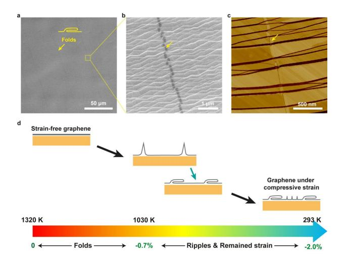
(a, b) SEM images and (c) AFM phase image of graphene folds in an adlayerfree single-crystal graphene film on a Cu(111) foil. (d) Schematic of the mechanism of graphene folds formation during the cooling process. Credit: Institute for Basic Science
