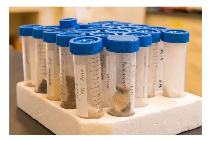
Chunks broken off of the concrete cylinders allowed for more analysis of internal conditions. Credit: University of Delaware
