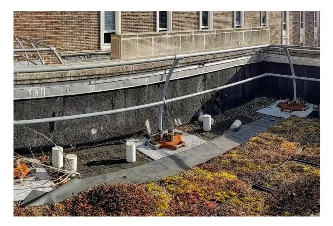
Forty concrete cylinders were placed on the roof of the University of Delaware's Spencer Lab to see how time and temperature changes would affect the bacterial communities within them. DNA samples were taken periodically and those samples were then sequenced and analyzed. Credit: University of Delaware
