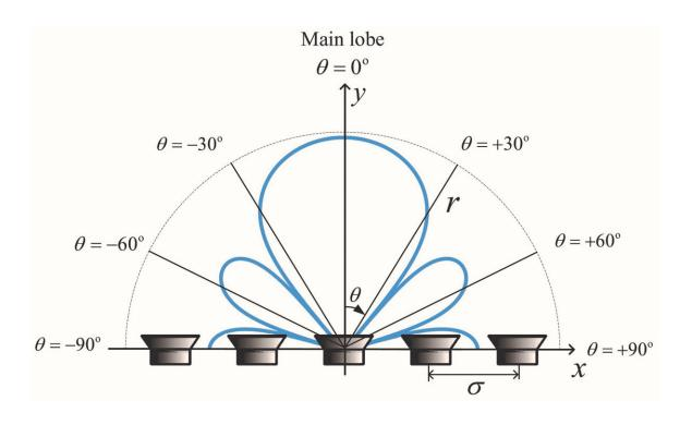
A compact speaker system designed to maximize the amount of sound moving toward zero degrees and minimize the sound leakage elsewhere. Credit: Wang et al.
