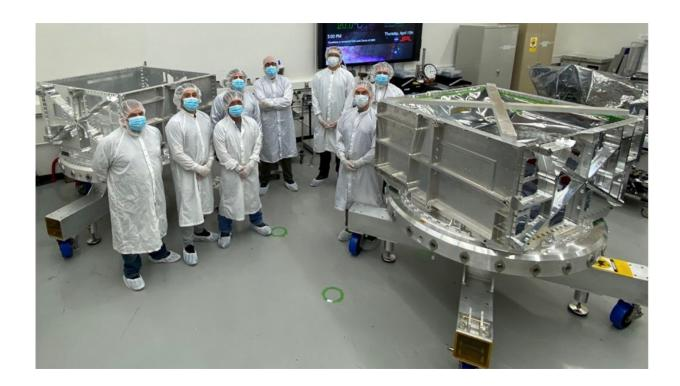
Engineers and technicians in a clean room at NASA's Jet Propulsion Laboratory in Southern California stand between the thick-walled aluminum vault and its duplicate (at rear) that they helped build for the agency's Europa Clipper spacecraft. As Europa Clipper orbits Jupiter, conducting flybys of its moon Europa to gather science data, the vault will protect the spacecraft's electronics from Jupiter's intense radiation. Credit: NASA/JPL-Caltech
