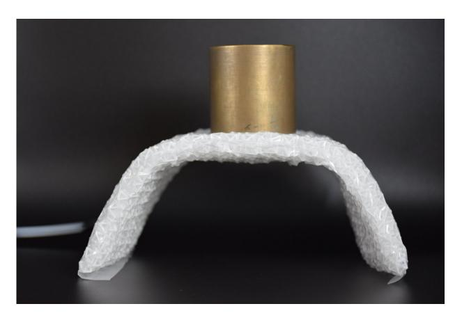
When stiffened, the new chain mail fabric developed by scientists from NTU Singapore and Caltech can withstand up to 50 times its own weight. Credit: NTU Singapore and Caltech
