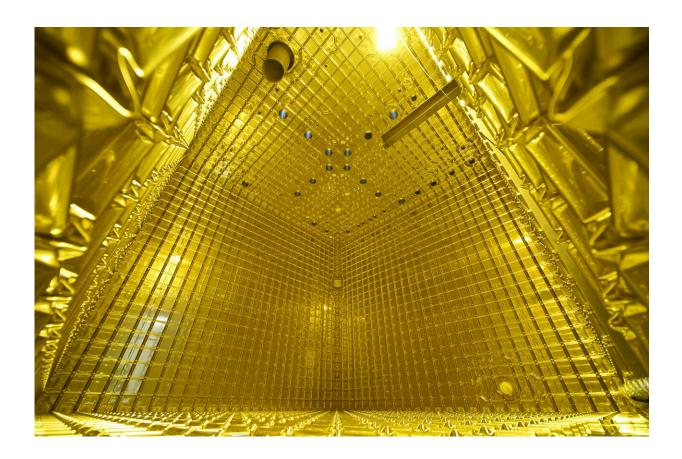
Inside a prototype liquid-argon time-projection chamber for the DUNE experiment. Credit: CERN
