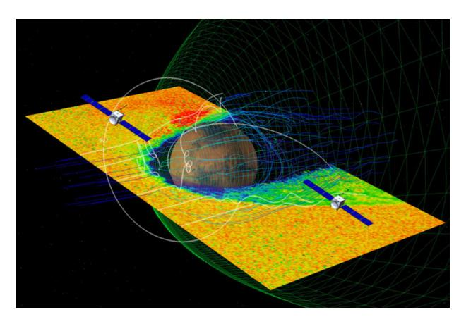
The twin ESCAPADE satellites should arrive at Mars in 2026, where they will circle the planet in complementary orbits to sample the hot ionized plasma (cross section in yellow and green) and magnetic fields (blue lines) to understand how Mars's atmosphere escapes into space. Credit: UC Berkeley / Robert Lillis
