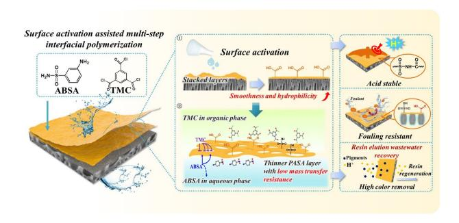
Schematic mechanism of preparation of acid-resistant nanofiltration membrane and its superior separation performance. Credit: CAO Yang
