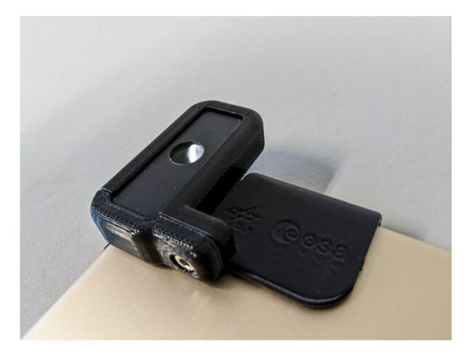
Preflight view of the hardware for Retinal Diagnostics, an investigation testing a commercially available ophthalmology lens to capture images of the human retina in space. Credit: DLR/EAC
