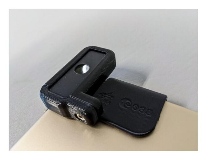
Preflight view of the hardware for Retinal Diagnostics, an investigation testing a commercially available ophthalmology lens to capture images of the human retina in space. Credit: DLR/EAC
