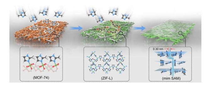
Schematic illustration of SAM assembly. Credit: DICP
