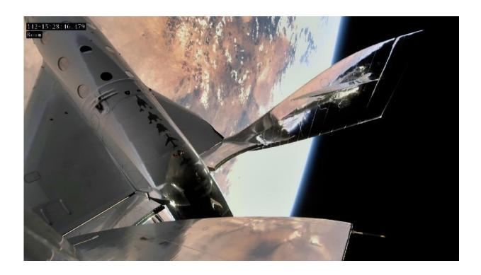
After climbing to 50,000 feet (15 kilometers), VSS Unity ignites its rocketpowered engine to ascend at Mach 3 beyond the 50 miles (80 kilometers) of altitude considered the edge of space.
