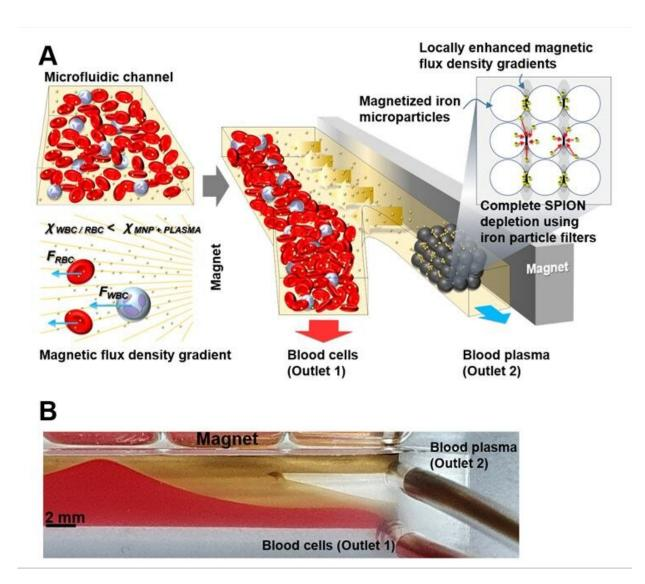
Figure 1. (A) A schematic illustration of the microfluidic device for blood plasma separation using diamagnetic repulsion of blood cells. (B) An image showing red blood cells diamagnetically repelled by permanent magnets. Credit:
