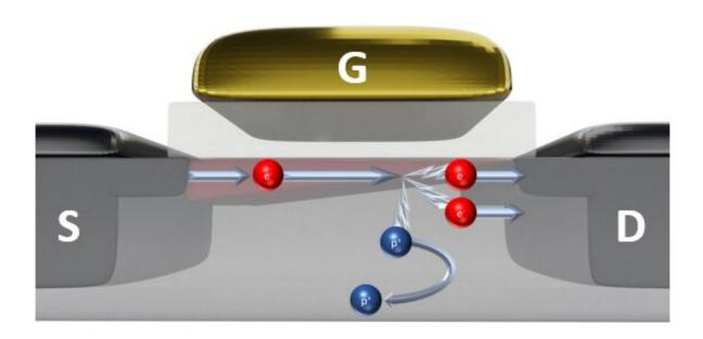
Through a process known as impact ionization, extra electric charges are generated inside transistors (as represented by the red electron and blue "hole" pair in this schematic n-channel metal oxide semiconductor field effect transistor or MOSFET). These pairs break up, and, at low temperatures, some of the positively charged holes are trapped in the transistor body, providing a way to store memory states. This impact ionization process underlies a novel proposed cryogenic memory. Credit: NIST
