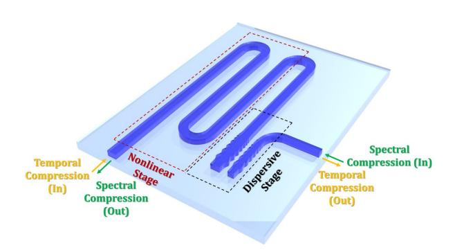
Schematic of the USRN compressor system. The system is comprised of separate nonlinear and dispersive stages. For spectral compression (SC), pulses enter the dispersive stage (DS) first before the nonlinear stage (NS), and for temporal compression (TC), pulses enter NS first before DS. Credit: SUTD
