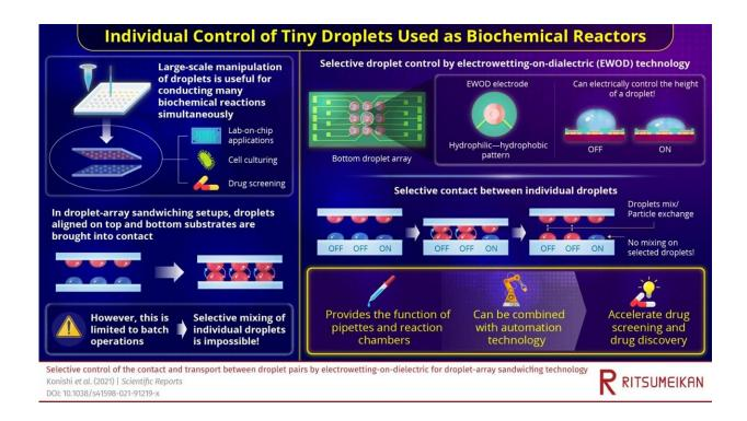
Controlling individual water droplets as biochemical reactors: Scientists from Ritsumeikan University, Japan develop a method to better manipulate tiny droplets in lab-on-a-chip applications for biochemistry, cell culturing, and drug screening. Credit: Ritsumeikan University, Japan
