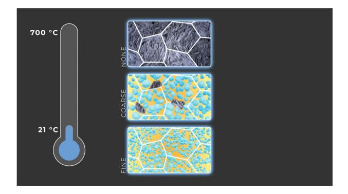
Nanoprecipitates suppressed phase transformation during thermal quenching and maintained the high-temperature face-centered cubic phase in a metastable state at room temperature. Credit: Michelle Lehman/ORNL, U.S. Dept. of Energy
