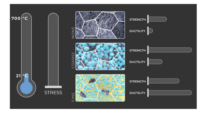
Subsequent stress during deformation transforms the material with coarse precipitates, making it stronger and more ductile, but does not change the one with fine precipitates. Credit: Michelle Lehman/ORNL, U.S. Dept. of Energy
