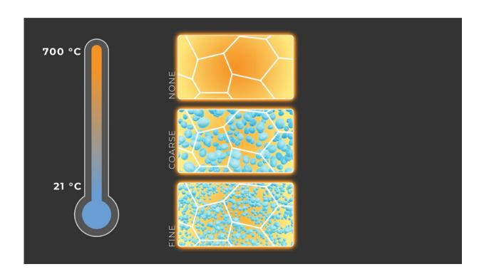
From top to bottom respectively, alloys were made without nanoprecipitates or with coarse or fine nanoprecipitates to assess effects of their sizes and spacings on mechanical behavior. Michelle Lehman/ORNL, U.S. Dept. of Energy. Credit: Michelle Lehman/ORNL, U.S. Dept. of Energy
