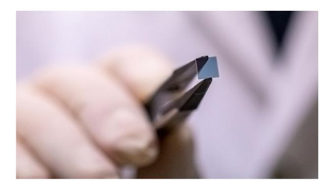
Handling a strontium and vanadium oxide (SrVO3) transparent film only few nanometers thick. Credit: ICMAB-CSIC
