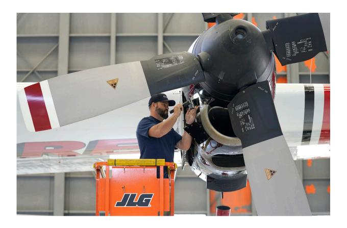
Aircraft Mechanic Cody Poole inspect one of the engines on a recently acquired C-130 aircraft, that will be used for firefighting, hangared at the California Department of Forestry and Fire Protection's Sacramento Aviation Management
