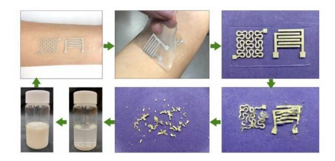
This image shows how the new recycling approach can take silver nanowires from a finished product (such as the flexible sensor patch in the top left) through the entire life cycle of the technology until it has been broken down for re-use (bottom left). Credit: Yong Zhu, North Carolina State University
