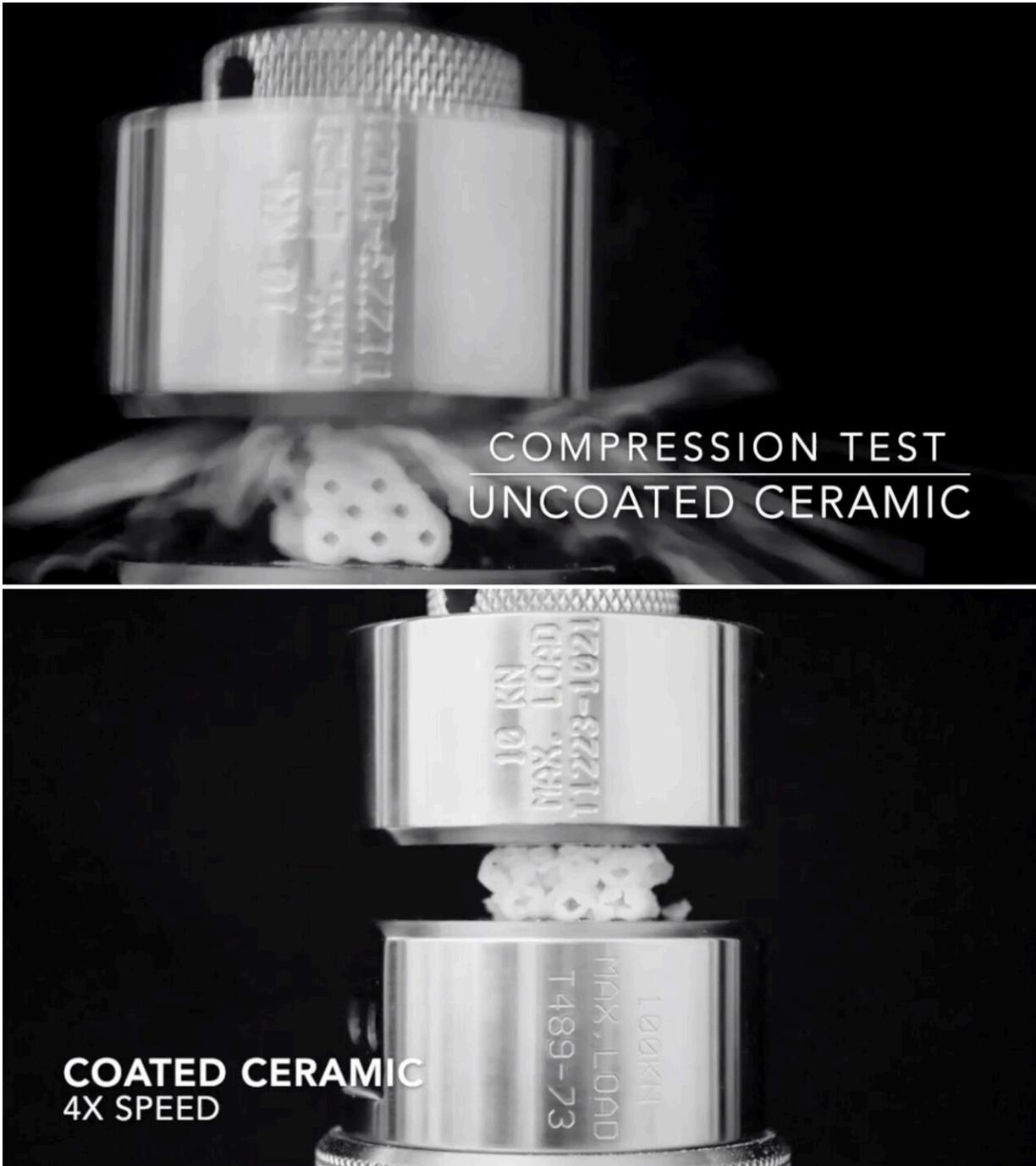
A compression test of 3D-printed schwarzites either coated or uncoated with a thin polymer shows how the polymer keeps the ceramic from shattering. The materials could be used wherever very strong but lightweight materials are needed. Credit: Ajayan Research Group/Rice University
