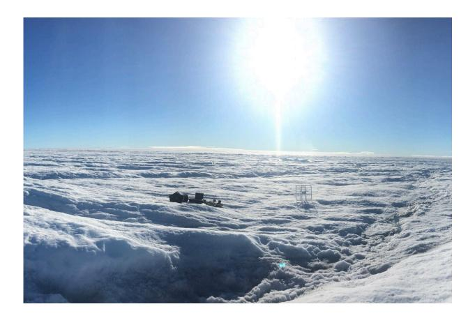
The experimental setup and test site at Store Glacier, Greenland. Researchers conceptualized a battery-powered receiver with an antenna placed on the ice that can measure ice thickness using the sun's radio waves. Credit: Sean Peters
