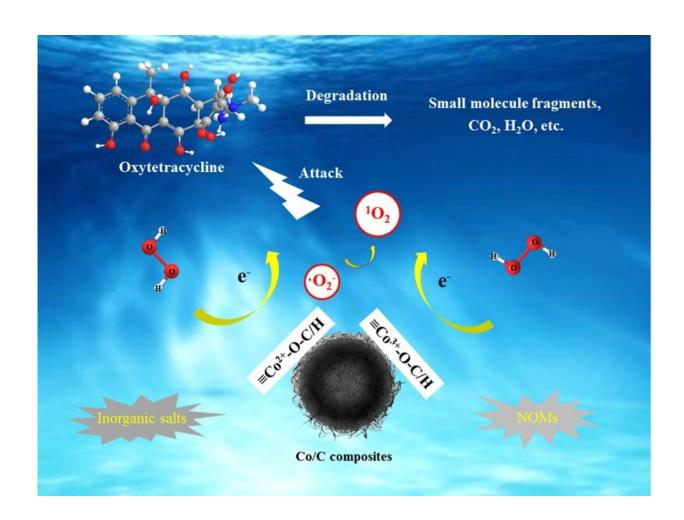
Mechanism diagram of the Co/C+H<sub>2</sub>O<sub>2</sub> system for selective degradation of the OTC pollutants. Credit: HONG Peidong
