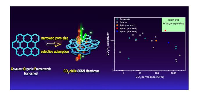
Illustration of superior CO2-selective COF nanosheet membrane for highperformance CO2/H2 separation. Credit: Peng Yuan
