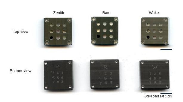
Front and back of each of the three, one-inch square plates. Tiny round windows allow the samples to be exposed to the harsh atmosphere in outer space. Credit: University of Illinois Dept. of Aerospace Engineering
