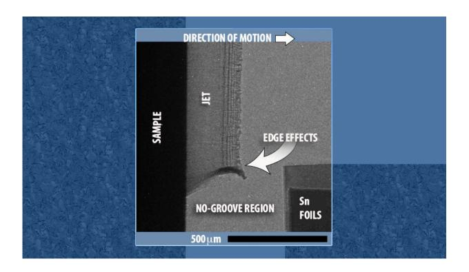
This representative dynamic image shows the base sample, emerging jet, nogroove control region and static calibration foils. Credit: Lawrence Livermore National Laboratory
