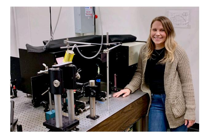
Hannah Rhoda with the resonance Raman spectroscopy equipment, which shoots a laser into a sample to obtain vibrational information from the exact site being
