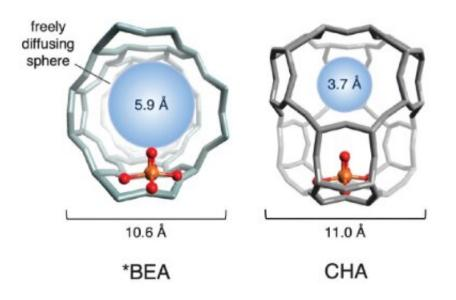
An illustration of the cage structures of two iron-based zeolites used in the study. The red and gold spheres (representing oxygen and iron, respectively) make up the active site. The cage structure, in gray, isformed of silicon, aluminum and oxygen. The blue sphere quantifies the size of the largest molecule that can diffuse freely in and out of the active site cage (the diameter of methane is ~4.2 Å). Credit: Benjamin Snyder
