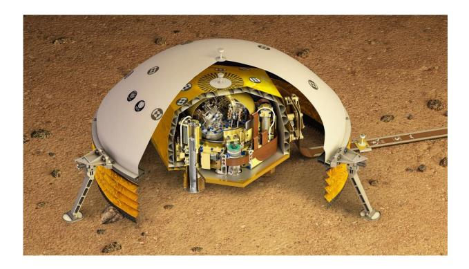
This artist's rendering shows a cutaway of the Seismic Experiment for Interior Structure instrument, or SEIS, which will fly as part of NASA's Mars InSight lander. SEIS is a highly sensitive seismometer that will be used to detect marsquakes from the Red Planet's surface for the first time. There are two layers
