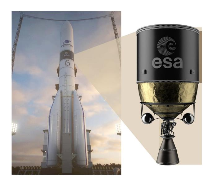
MT Aerospace and ArianeGroup signed contracts with ESA on 14 May 2019 to develop Phoebus, a prototype of a highly-optimised black upper stage. Rocket upper stages are commonly made of aluminium but switching to carbon
