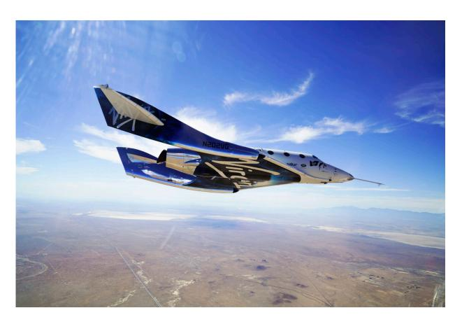
This May 29, 2018 photo made available by Virgin Galactic shows the company's VSS Unity on its second supersonic flight. After reaching nearly 50,000 feet (15,000 meters), Unity will be released from the specially designed aircraft Mothership Eve, and drop for a moment or two before its rocket motor ignites to send the craft on a steep climb toward space. Credit: Virgin Galactic via AP
