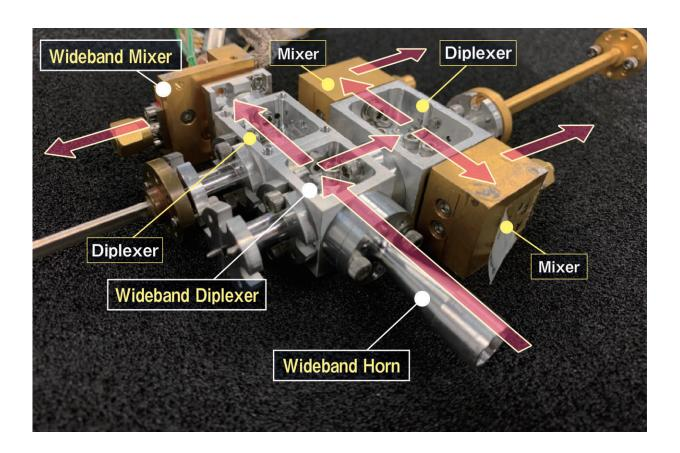
Newly developed radio receiving system. The radio waves collected by the antenna are directed to the receiver through the horn at the lower left of the photo and follow the path indicated by the arrow to be output. Credit: Osaka Prefecture University
