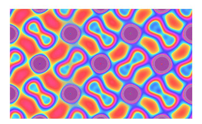
As a compound of manganese sulfide is compressed in a diamond anvil cell, it undergoes dramatic transitions. In this illustration, the interaction between the manganese (Mn) atomic ions (purple circles) and disulfur ( $S_2$ ) molecular ions (figure 8s) increases from left to right until the overlap is significant enough to make the system metallic. Credit: Dean Smith, Argonne National Lab
