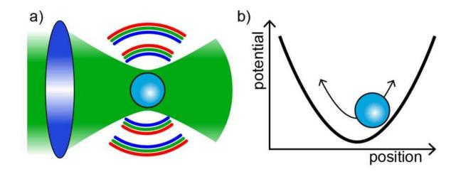
A nanosphere is made to hover by focused laser light (a). The laser light acts as a trap in which the sphere can oscillate back and forth (b). Electric fields are used to slow down that motion. Credit: ETH Zurich
