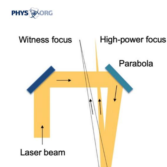
At the heart of the Berkeley Lab innovation is a wedge-shaped optic with a 99% reflective front surface for the main beam, and a wedged rear surface to reflect a low-powered witness beam. Both reflected beams are brought to a focus at nearly the same distance along near-identical paths, so the witness beam undergoes the same motions as the main beam. Credit: Berkeley Lab
