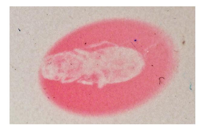
After exposure to X-rays, the hackmanite film is left with an X-rayed image of the ant. The photo has been taken with a DSLR camera. Credit: Sami Vuori
