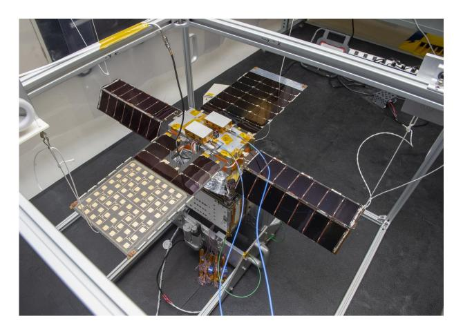
NASA's NEA Scout spacecraft in Gravity Off-load Fixture, System Test configuration at NASA's Marshall Space Flight Center in Huntsville, Alabama. Credit: Jet Propulsion Laboratory
