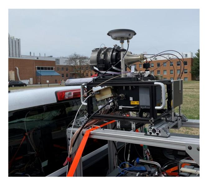
The hazard detection lidar system. Credit: NASA
