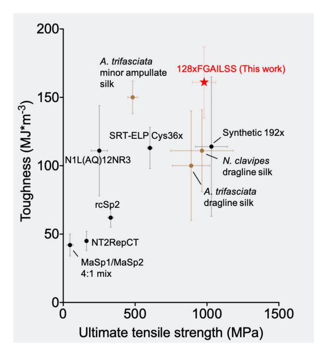
This chart compares the toughness and strength of different natural and recombinant silk fibers. In red is the polymeric amyloid fiber developed in Fuzhong Zhang's lab. Credit: Washington University in St. Louis/Jingyao Li
