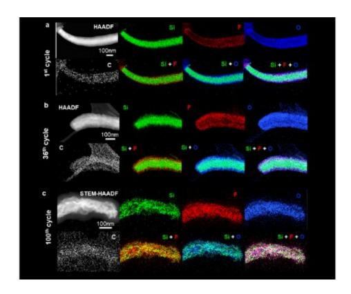
Cryo-STEM imagery showing the structural and chemical evolution of silicon and the solid-electrolyte interphase (SEI) layer. After the 36th cycle to the 100th cycle the silicon nanowire expands and becomes irregular, mingling with the SEI to form a soft composite structure. Credit: Jennifer M. Mccann
