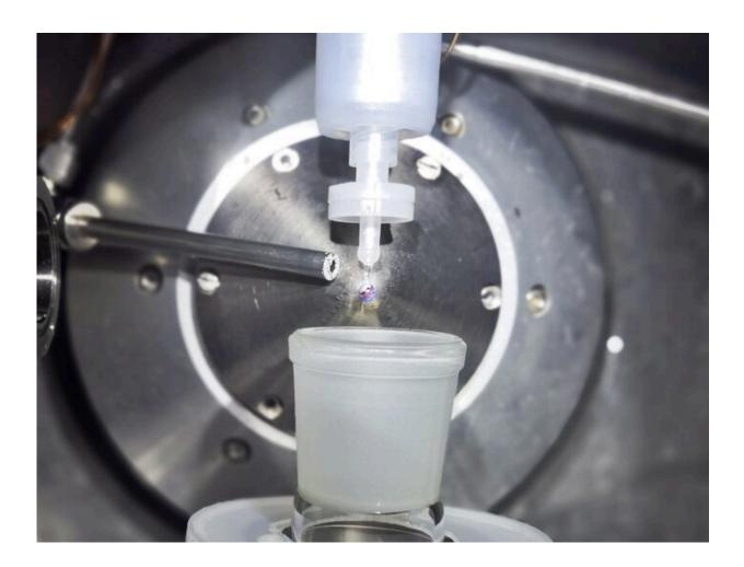
In the sample chamber, the NaK alloy drips from a nozzle. As the droplet grows, water vapor flows into the sample chamber and forms a thin skin on the drop's surface. Credit: HZB
