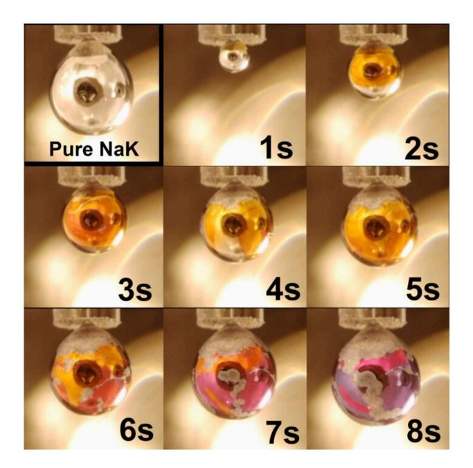
The first image shows a pure drop of sodium-potassium alloy; in the next images, we see the drop exposed to the action of the water vapor at 10-4 mbar. A layer of water forms on the drop, in which electrons liberated from the metal dissolve, giving it a golden metallic sheen. Credit: Phil Mason / IOCB Prague
