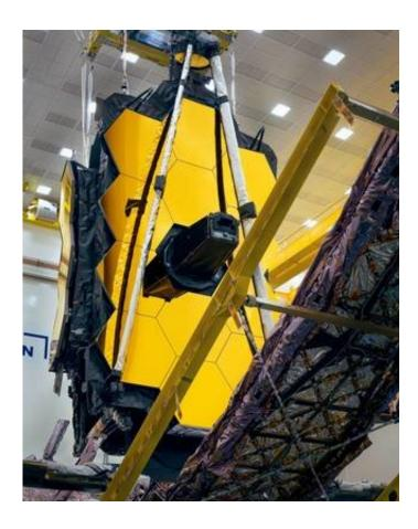
After the removal of the James Webb Space Telescope's "lens cap" engineers were freed to fold up the long support structures that keep the observatory's sunshield safe and secure during transport and deployment. Credits: NASA/Chris Gunn
