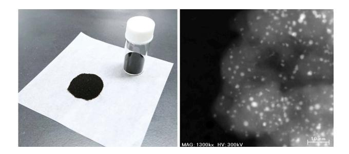
The newly developed catalyst in powder form (left) and under a transmission electron microscope (right; Photo: Shinya Furukawa). Credit: Shinya Furukawa
