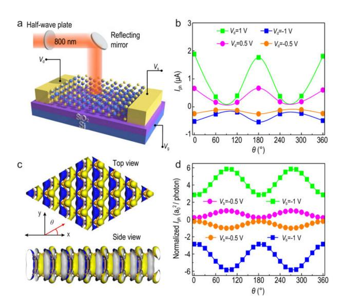
(a) The configuration for angle-dependent transport behavior determination. (b) Angular dependence of the photocurrent of the device at Vds = 0.5 V and Vds = 1 V, respectively. (c) Top-view and side-view of the contributing orbital to the
