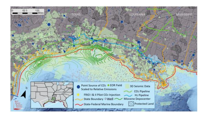
A map of Gulf Coast infrastructure that could help in developing a carbon capture and storage hub in the region. The infrastructure includes commercial CO2 pipelines, hydrogen pipelines, and industrial CO2 emission sources. Credit: Meckel et al. / The University of Texas at Austin.
