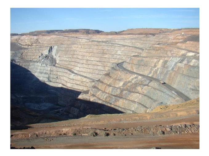
A giant gold deposit in W. Australia (SuperPit). Pyrite and arsenopyrite are the major ore minerals concentrating invisible gold together with arsenic. Credit: Gleb Pokrovski
