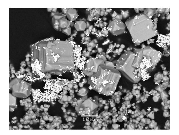
Scanning electron microscopy photomicrograph showing gold microparticles (bright color) deposited with pyrite crystals from a hydrothermal solution in a laboratory experiment. Such experiments simulate the formation of gold deposits in nature. Credit: Maria Kokh and Gleb Pokrovski
